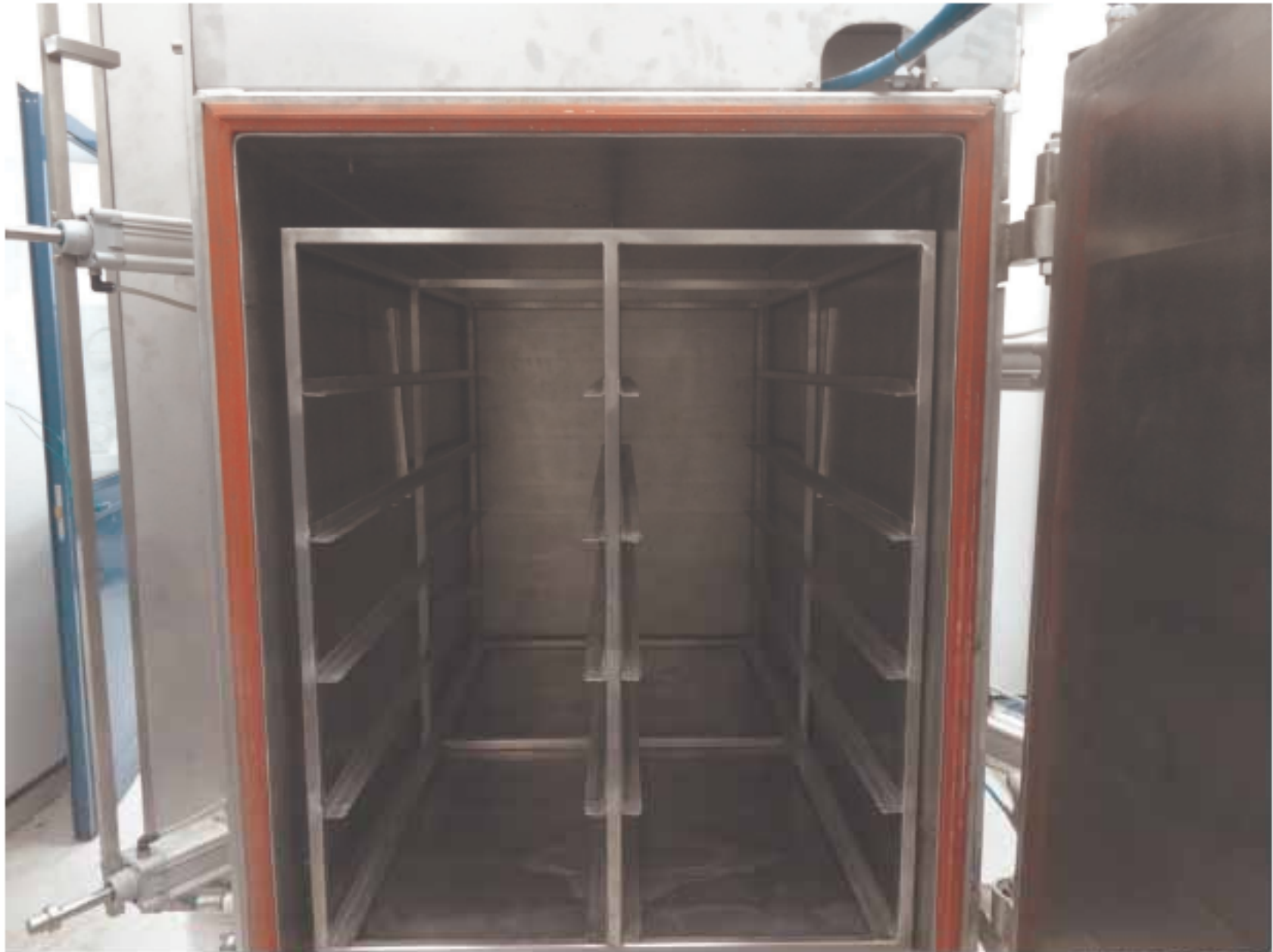
1.6 M3 STERILIZER – TRAY CARCASS – SKELETON INTERIOR VIEW
